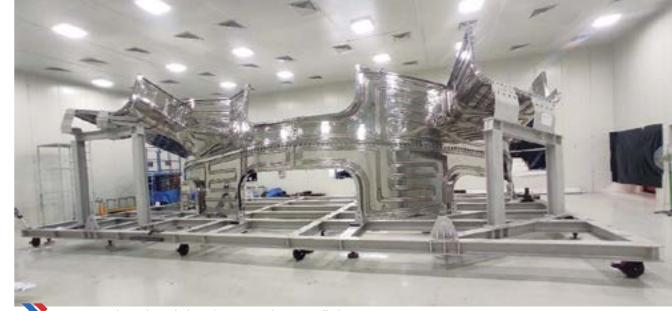
VVTS Repair work carried out for ITER Project at Savli Plant
